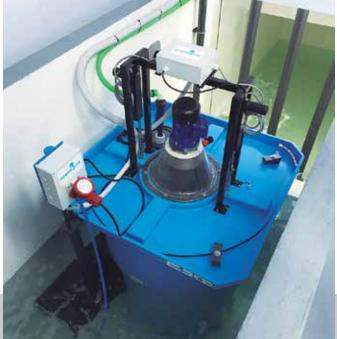
The automatic adjustment of the foam formation minimizes the water consumption in a recirculation system and always guarantees a correct purification.
